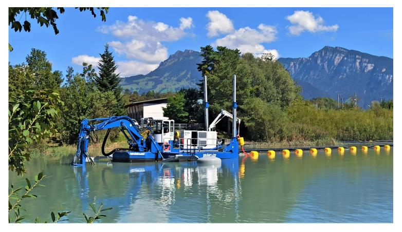
**DRSP** (Multi-Purpose series) represents a step over on approach of dredging technique. The extreme mobility in any kind of swamp, together with the **full floatability**, allow to reach the most remote locations otherwise impossible to get with any other equipment.
